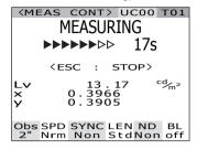
(Continuous measurement/when measurement time is short)
